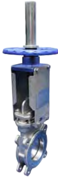
BKGV-D LUGGED AS2129 TABLE D KNIFE GATE 316 Stainless Steel EPDM seat 1000Kpa 100mm to 600mm
